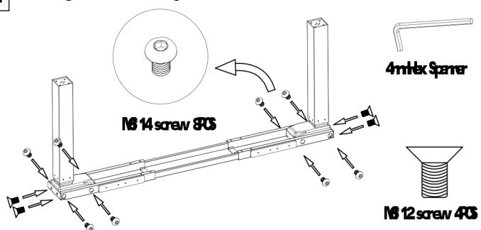
3 Attach feet to the legs using 8 of M8 16 screw, attach the 4 of leading foot pads to the feet by hand
