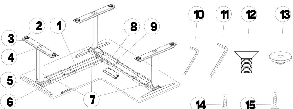
1 Loosen the 4 screws of bar using 4W hex spanner, adjust the bar to proper position to fit the desktop
