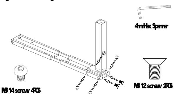
6 Attach feet to the legs using 4 of M8 16 screw, attach the 2 of leading foot pads to the feet by hand
