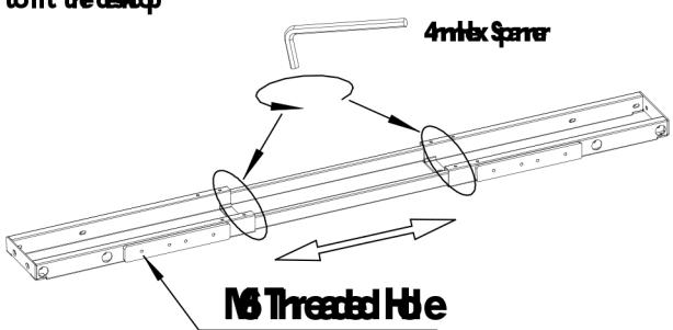
2 Attach legs to the bar using 8 of M8 14 screw and 4 of M8 12 screw
