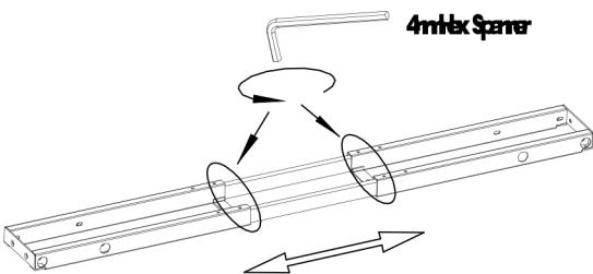
5 Attach legs to the bar using 4 of M8 14 screw and 2 of M8 12 screw
