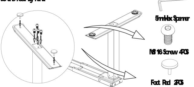
7 Attach the bar to the bar using 2 of M8 10 screw
