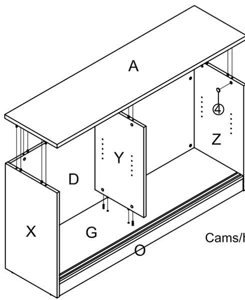
Cams/holes on the panel Y to face to panel X.
