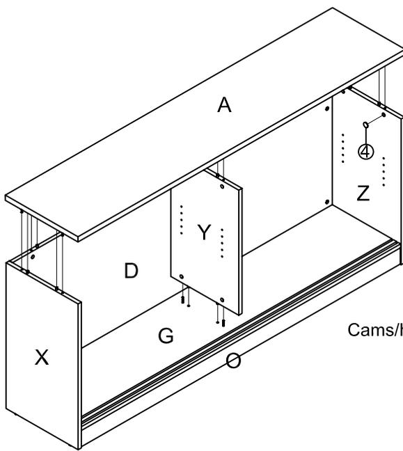
Cams/holes on the panel Y to face to panel X.
